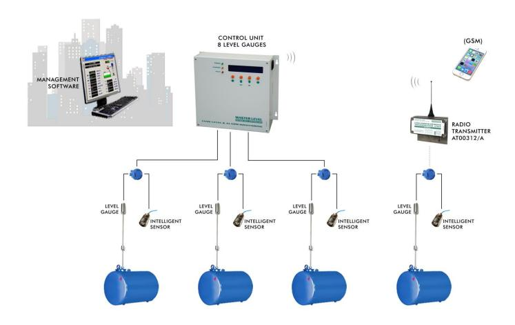
Level measurement and leakage alarm monitoring control unit for tanks, piping and wells. Management of 8 level guages and 16 leakage alarm sensors, 4/8 on/off inputs and up to 8 relays with programmable-event outputs. It can be connected to other 4 devices to extend the level, alarm and relay control and to allow interfacing with main control systems installed on refuelling stations.
